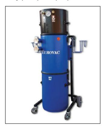
The Eurovac II portable is powered by compressed air being forced through a venturi to create a powerful vacuum. Using compressed air eliminates the chance of a dust or gas explosion as there is no sparking motor. To meet NFPA codes, the system is grounded and the vacuum hoses and cuffs are static conductive.
