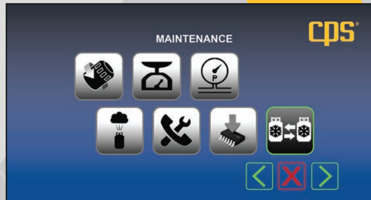
Refrigerant Change Screen: select Refrigerant Change key (highlighted) and follow onscreen instructions to change refrigerant.
