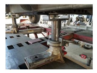
Use of these adapters along with the F.A.S.T accessories and Universal base stands allow a technician to quickly set up a vehicle for measuring. The rail saddle plates are also useful when used for measuring and they are wide enough to be used on the wider frames on some vehicles.
