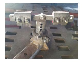
This adapter allows the use of F.A.S.T. accessories with Universal base plates
